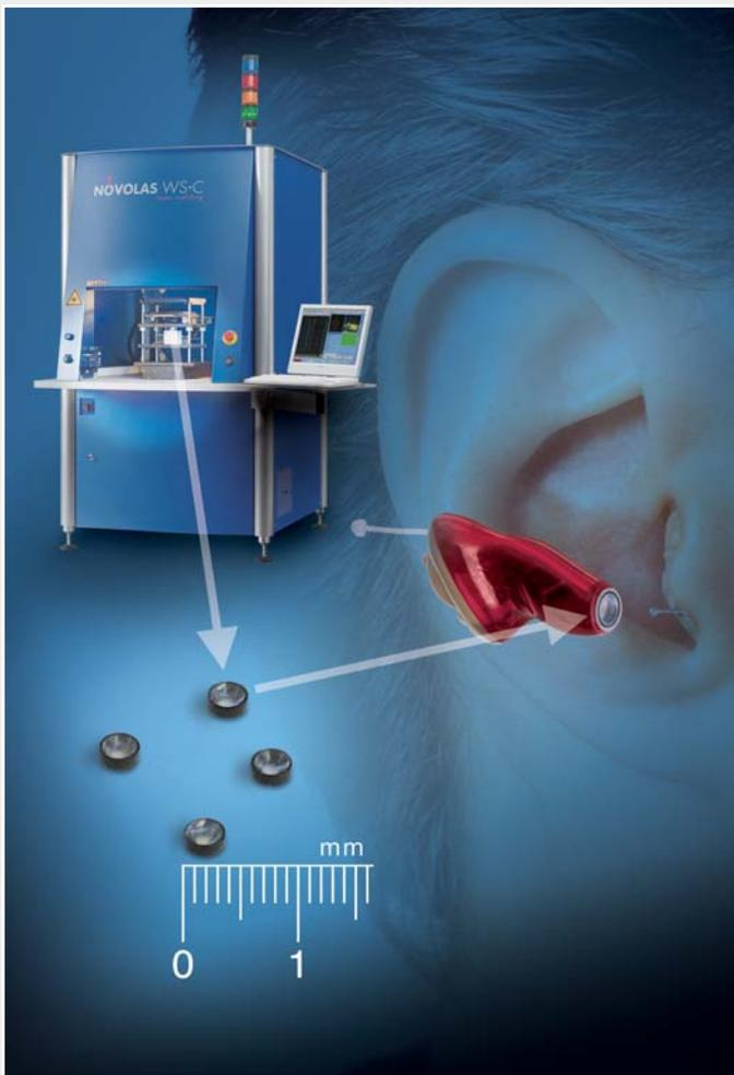
*The diaphragm is welded upon the cerumen protection on a Leister WS (work station).*
